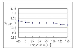
Figure 7. Stop Threshold Voltage
