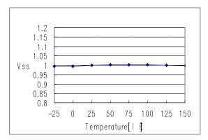
Figure 13. Soft Start Voltage
