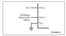
Figure 4. External Clock Drive Configuration
