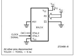
Figure 6.  $I_{CC}$  Test Condition, Active Mode
