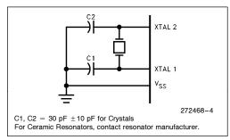
Figure 3. Oscillator Connections
