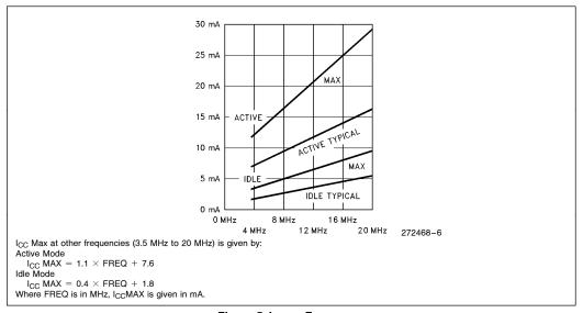
Figure 5. I<sub>CC</sub> vs Frequency
