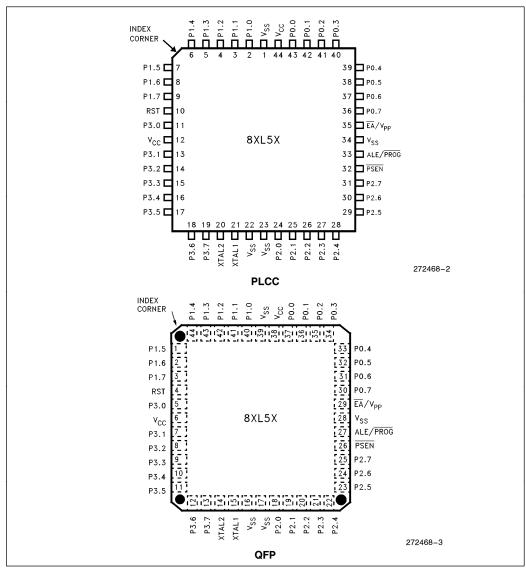
Figure 2. Pin Connections
