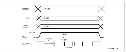
Figure 11. Programming Signals Waveforms
