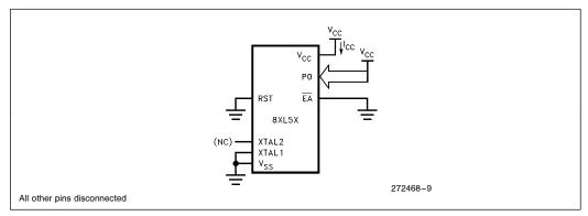
Figure 8. I<sub>CC</sub> Test Condition, Power Down Mode.  $V_{CC} = 2.7 V$  to 3.6 V.
