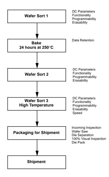
Figure 1. AMD KGD Product Test Flow
