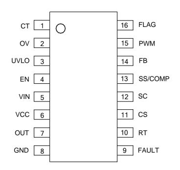
Figure 1. Pin Configuration of AP3041 (Top View)
