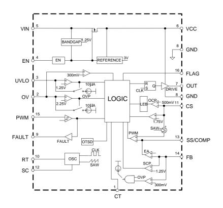
Figure 2. Functional Block Diagram of AP3041
