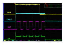
Figure 6. Dimming Minimum on Time Control
