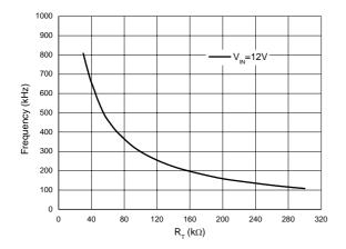
Figure 5. Frequency vs. R<sub>T</sub>
