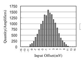
Figure (a) Input Offset Voltage Distribution
