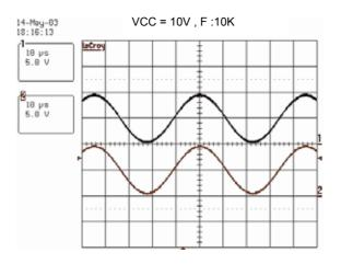
Figure (c) Rail to Rail Capability
