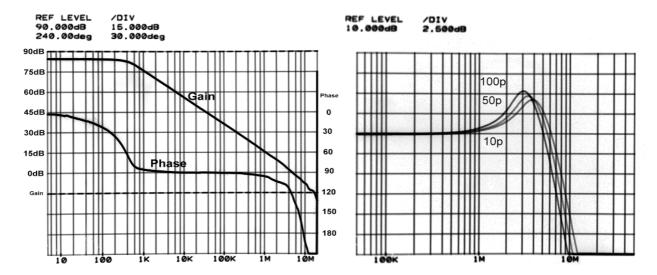
Figure (g) Open Loop Gain & Phase vs. Frequency
