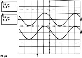
Figure 1. Operation with Rail-to-Rail Input and Output
