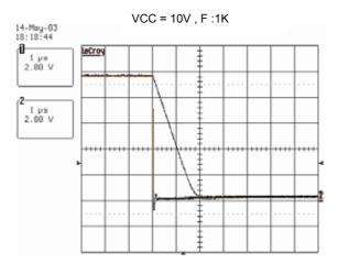
Figure (e) Large Signal Transient Response
