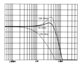
Figure (h) Frequency Response for Various R<sub>L</sub>
