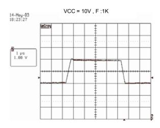
Figure (f) Small Signal Transient Response
