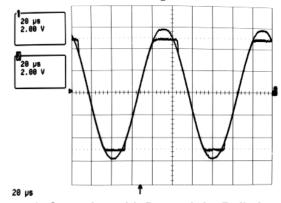
Figure 2. Operation with Beyond-the Rails Input
