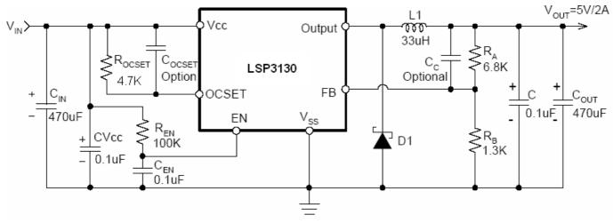
Note1:CIN/COUT can be Electro capacitor or Tan capacitor; The typical CIN Electro capacitor is 470uF/35V, the typical CIN Tan capacitor is 100uF/35V; The typical Cout Electro capacitor is 470uF/16V, the typical Cout Tan capacitor is 22uF/16V;
