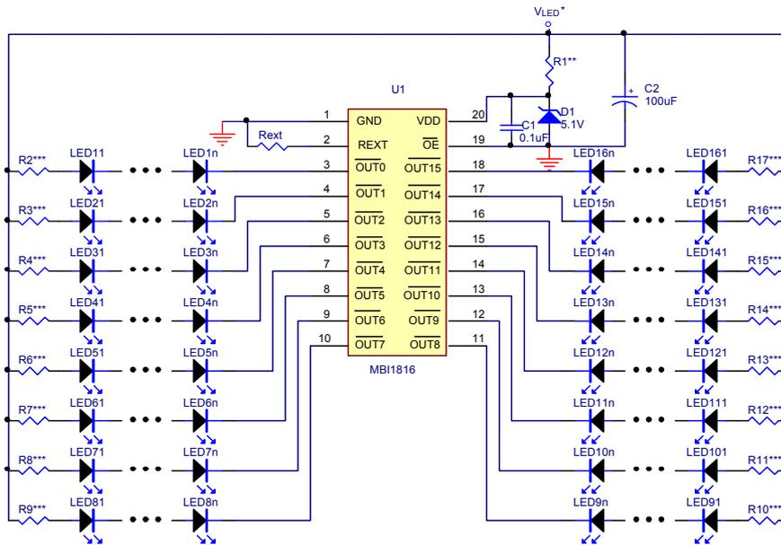
\*  $V_{LED} > V_{DS} + V_{F,LED} \times n$ ;  $V_{F,LED}$ : Forward voltage of LED; n: LED count
