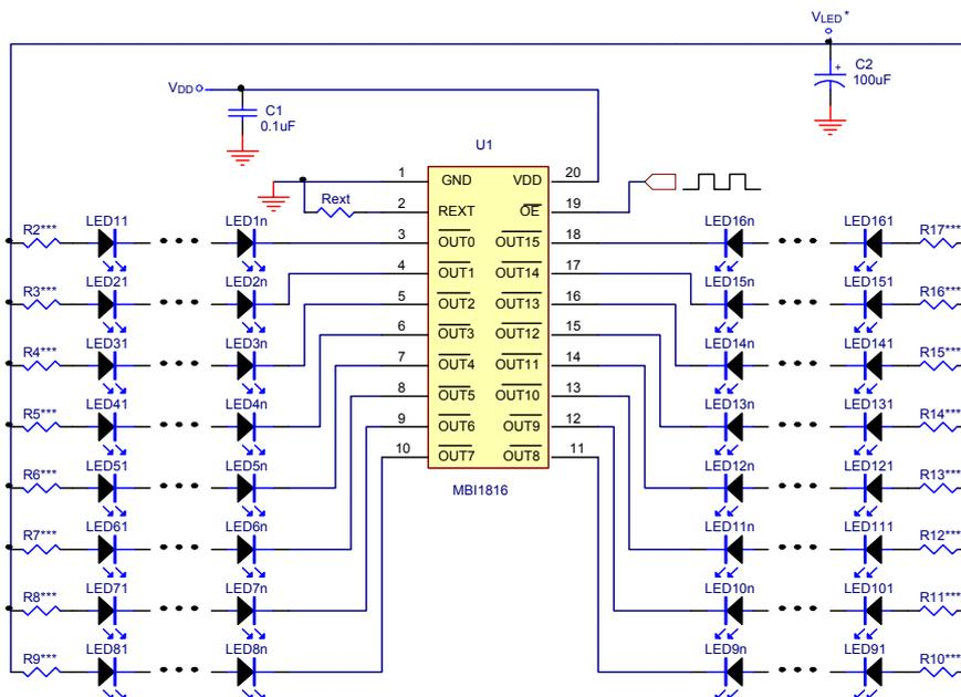
\*  $V_{LED} = V_{DS} + V_{F,LED} \times n$ ;  $V_{F,LED}$ : Forward voltage of LED; n: LED count
