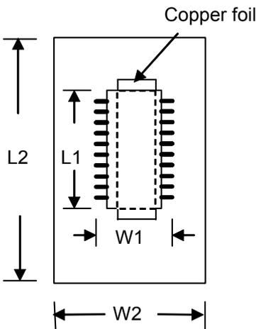
The PCB area  $L2 \times W2$  is 4 times of the IC's area  $L1 \times W1$ .
