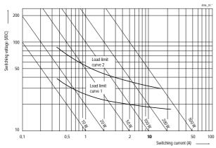
Load limit curve 1: arc extinguishes during transit time (changeover contact)
