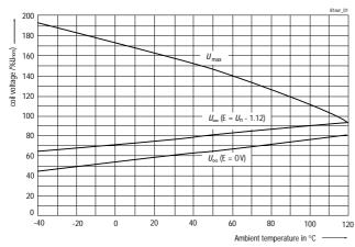
Does not take into account the temperature rise due to the contact current
