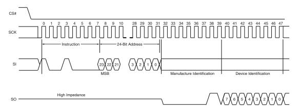
Figure 9.10 Read-ID (RDID) Command Timing Diagram
