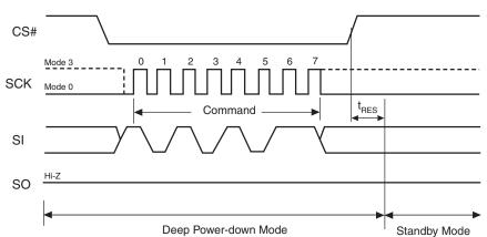
Figure 9.23 Release from Deep Power-Down (RES) Command Sequence
