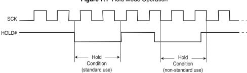
Figure 7.1 Hold Mode Operation
