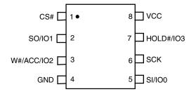
Figure 2.3 8-contact USON (5 x 6 mm) Package
