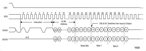
Figure 9.5 DUAL I/O High Performance Read Instruction Sequence
