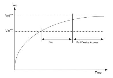
Figure 11.1 Power-Up Timing Diagram
