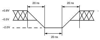
Figure 14.2 Maximum Positive Overshoot Waveform
