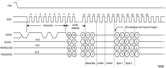
Figure 9.7 QUAD I/O High Performance Instruction Sequence
