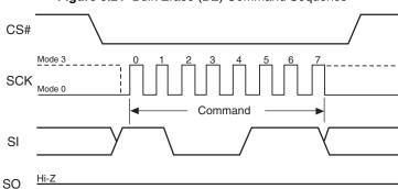
Figure 9.21 Bulk Erase (BE) Command Sequence
