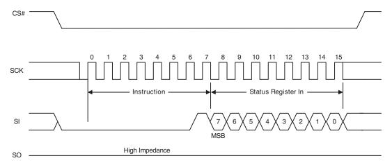
Figure 9.15 Write Registers (WRR) Instruction Sequence – 8 data bits
