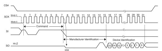
Figure 9.9 Read Identification (RDID) Command Sequence and Data-Out Sequence
