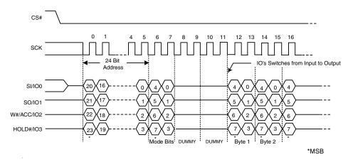
Figure 9.8 Continuous QUAD I/O High Performance Instruction Sequence
