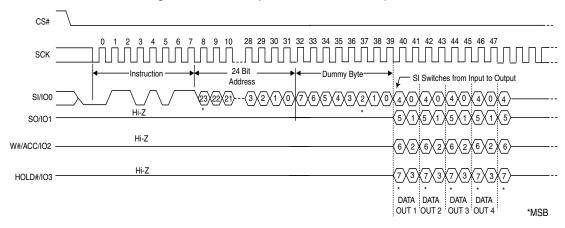
Figure 9.4 Quad Output Read Instruction Sequence
