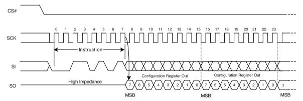
Figure 9.14 Read Configuration Register (RCR) Instruction Sequence
