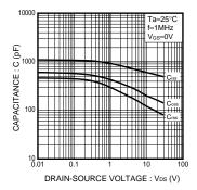
Fig.1 Typical Capacitance vs. Drain-Source Voltage
