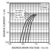
Fig.6 Source Current vs. Source-Drain Voltage
