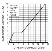
Fig.3 Dynamic Input Characteristics
