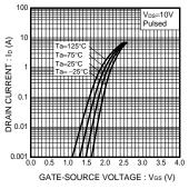
Fig.4 Typical Transfer Characteristics
