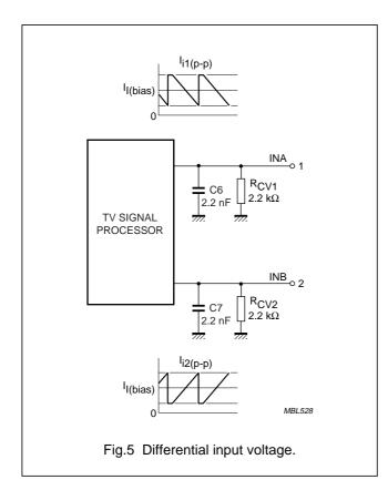
Values for these currents are, for instance  $I_{i(bias)} = 400 \mu A$ ;  $I_{i1(p-p)} = I_{i2(p-p)} = 475 \mu A$ .
