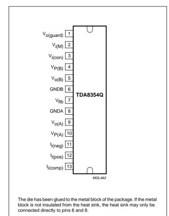
Fig.2 Pin configuration.
