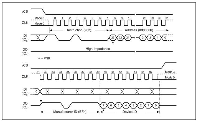
Figure 29. Read Manufacturer / Device ID Instruction (SPI Mode)
