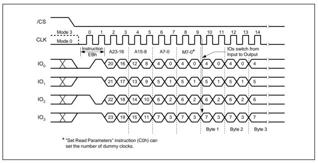
Figure 15c. Fast Read Quad I/O Instruction (Initial instruction or previous M5-4≠10, QPI Mode)
