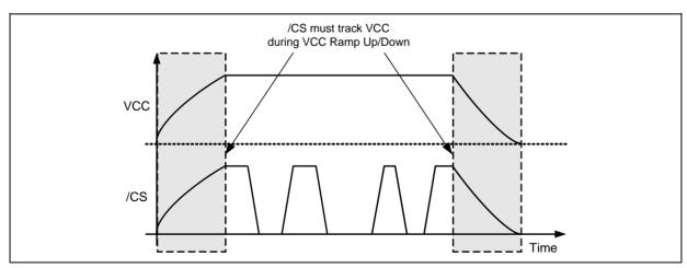
Figure 43b. Power-up, Power-Down Requirement
