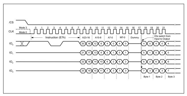
Figure 16a. Word Read Quad I/O Instruction (Initial instruction or previous M5-4 ≠ 10, SPI Mode only)
