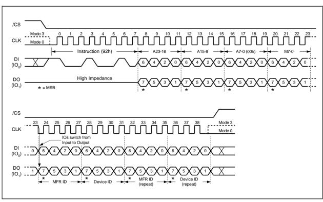
Figure 30. Read Manufacturer / Device ID Dual I/O Instruction (SPI Mode only)
