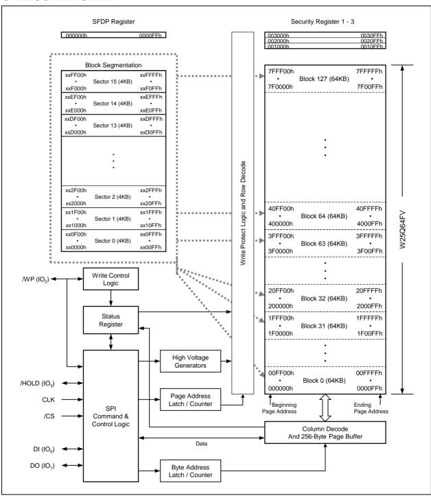
Figure 2. W25Q64FV Serial Flash Memory Block Diagram
