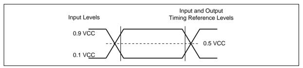
Figure 44. AC Measurement I/O Waveform
