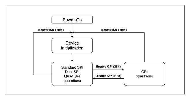
Figure 3. W25Q64FV Serial Flash Memory Operation Diagram
