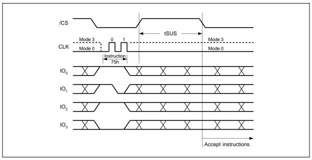
Figure 25b. Erase/Program Suspend Instruction (QPI Mode)
