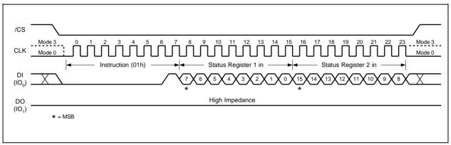
Figure 9a. Write Status Register Instruction (SPI Mode)
