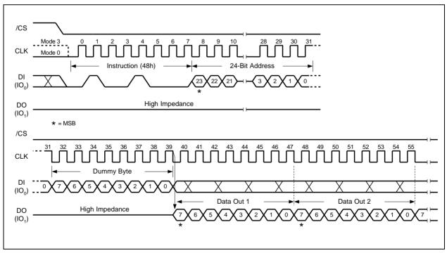
Figure 37. Read Security Registers Instruction (SPI Mode only)
