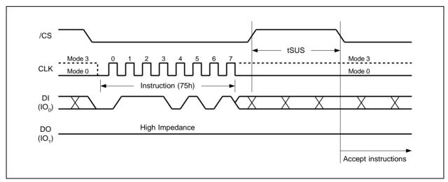
Figure 25a. Erase/Program Suspend Instruction (SPI Mode)
