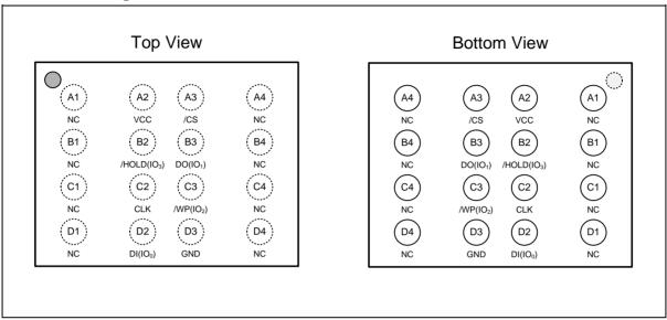
Figure 1e. W25Q64FVBall Assignments, 16-ball WLBGA (Package Code BY)
