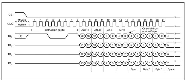
Figure 17a. Octal Word Read Quad I/O Instruction (Initial instruction or previous M5-4 ≠ 10, SPI Mode only)
