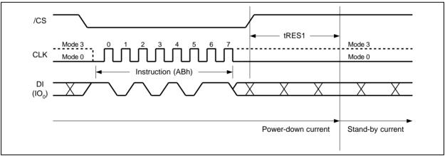
Figure 28a. Release Power-down Instruction (SPI Mode)
