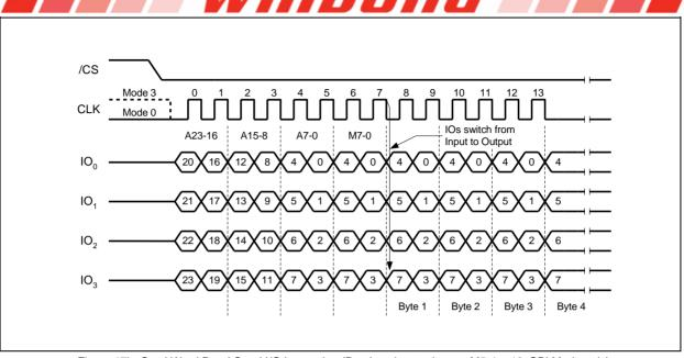
Figure 17b. Octal Word Read Quad I/O Instruction (Previous instruction set M5-4 = 10, SPI Mode only)
