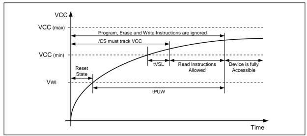
Figure 43a. Power-up Timing and Voltage Levels
