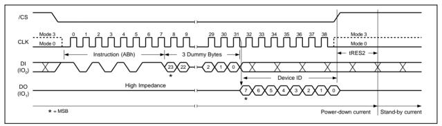
Figure 28c. Release Power-down / Device ID Instruction (SPI Mode)
