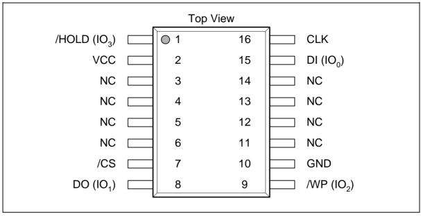
Figure 1d. W25Q64FV Pin Assignments, 16-pin SOIC 300-mil (Package Code SF)
