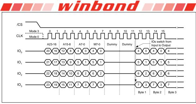
Figure 15b. Fast Read Quad I/O Instruction (Previous instruction set M5-4 = 10, SPI Mode)
