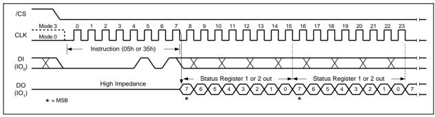
Figure 8a. Read Status Register Instruction (SPI Mode)
